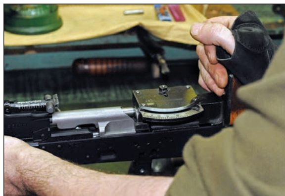
After bolts are carefully hand and fit to each Beryl rifle, they're individually checked with a gauge that measures the force required to close and lock the bolt.
