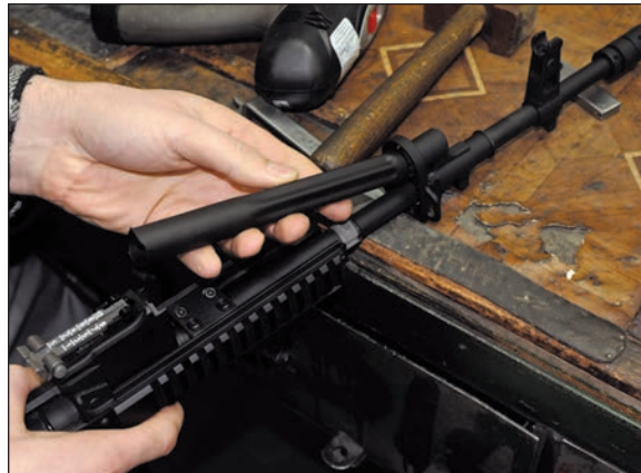
After installing a railed fore-end on a Beryl, a worker slides the gas tube into position. Note how the fore-end is locked in place by a retainer.
